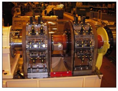
the unit is in operation and carrying normal load. The arms are 100% tin plated. The rigging is anchored to the steel base through an electrically insulating anchoring system.
