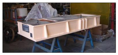
prior to shipping. The base, itself, will be bolted and doweled to the existing foundation sole plate as a part of the field installation and alignment and supports the above components. Additionally, it acts as an air duct for cooling medium.
