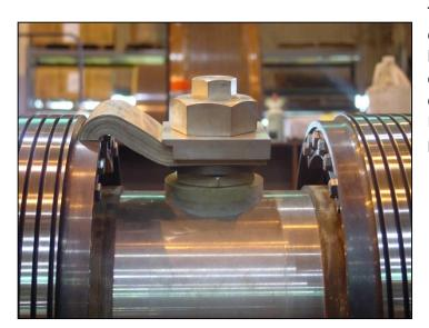
The flex lead connectors are comprised of a stack of copper laminations. They make the connection between the collector rings and radial studs. Each lamination is 100% tinplated.
